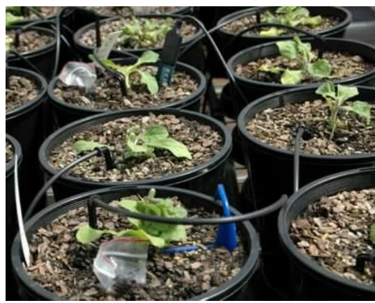
Aquaspy in foreground and ECH2O in background used to assess moisture content within rootzone environments to allow irrigation scheduling
