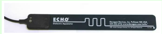
Soil moisture sensors - Blue is Aquaspy and green is the ECH2O
